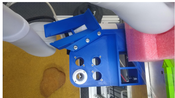
Figure 8. Top view of 3D printed RSA and RRB with one RSTA slot filled
